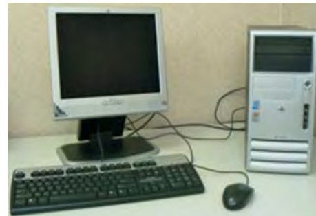
Fig. 3.20: System unit connected with basic input and output devices
