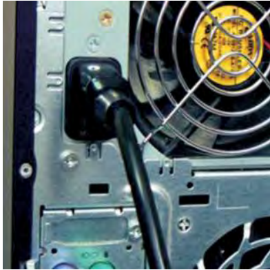
Fig. 3.18: Plug Power Supply Cord into System Unit and Power Supply Cable into Power Strip
